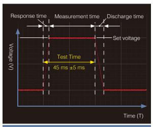
Applied Voltage Waveform at Fastest Test Time
